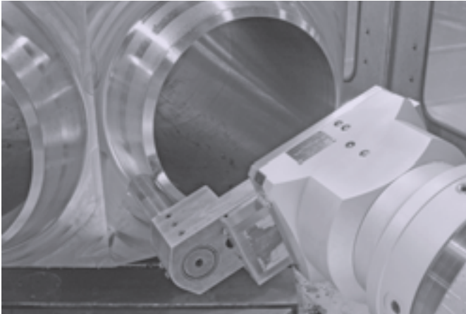
ZX-420 Facing/Contouring Tool machines O.D. tapers on a 24 in. "Y" block.
